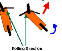
Whether the engine is driving the rear tire or not, because the bike is not simply 'dragging/scuffing' the rear tire forward with it (because the tire is now rotating), the bike begins to move faster (actually, is slowing more slowly) in the direction pointed to by the front tire. At the same time, because full traction has been regained, the sliding movement of the rear end of the bike comes to an abrupt end. And what next happens is the high-side!
